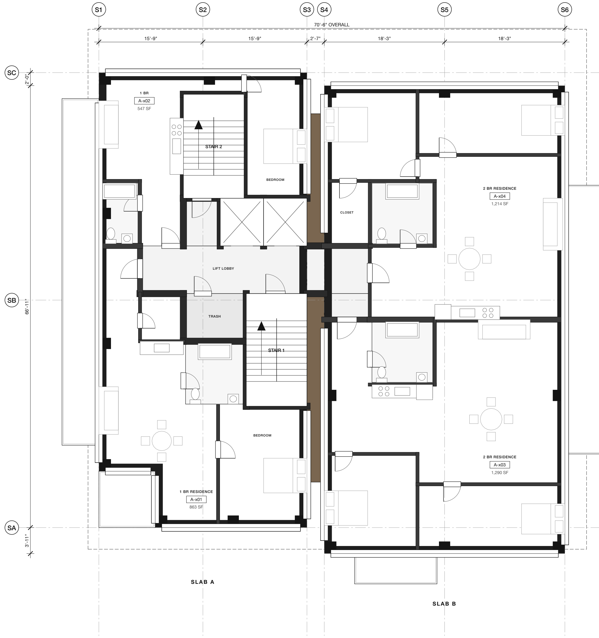
3 TYPICAL LEVEL PLAN, LEVELS 3-21 SCALE: 1:100
